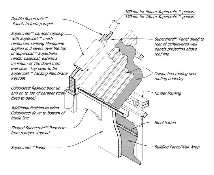
**NOTE:** Where the capping overhangs the wall as shown, the Supercoat™ Tanking Membrane System shall return under the overhang and down the vertical sides of the capping, back to the wall face. Where the capping is flush with the wall face, the Supercoat™ Tanking Membrane System shall return 100mm down the wall face. Please see Supercoat™ Waterproofing Systems Technical Manual (SWSTM 2013) located at www.supercoat.co.nz
